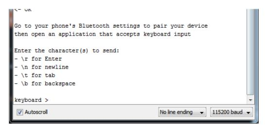
To send keyboard data, type anything into the textbox at the top of the Serial Monitor and click the **Send** button.
