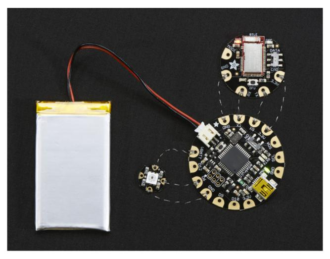
Sewing the Flora BLE to a Flora is very straight-forward: the four required pads line up so just sew those in short straight lines from one module to another. the **MODE** pad is not required for most uses so you can leave that unconnected.
