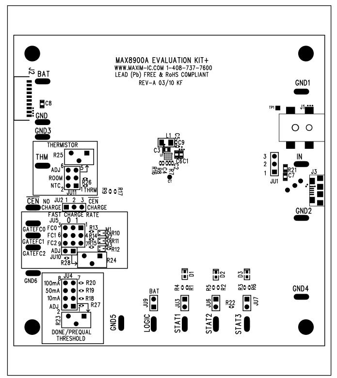
Figure 10. MAX8900A EV Kit Component Placement Guide—Top Layer
