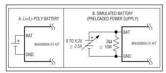
Figure 2. Battery Options for Evaluating the MAX8900A EV Kit
