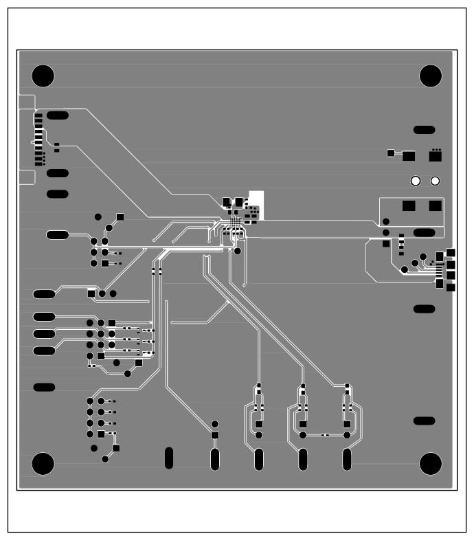
Figure 11. MAX8900A EV Kit PCB Layout—Top Layer
