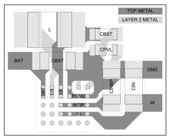
Figure 4. Power PCB Layout Example
