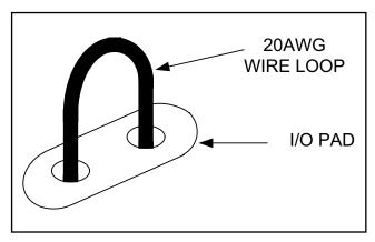
Figure 7. Wire Loop in I/O Pad Provides Convenient Attach
