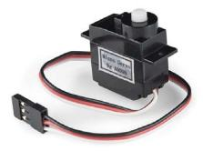
Unlike the action of most motors that continuously rotate, a servo motor can rotate to and hold a specific angle until it is told to rotate to a different angle. You can control the angle of the servo by sending it a PWM (Pulse Width Modulation) pulse train; the PWM signal is mapped to a specific angle from 0 to 180 degrees.
