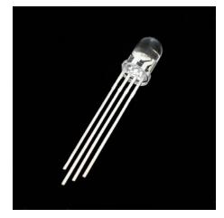
The Red Green Blue (RGB) LED is 3 LEDs in one. The RGB has four pins with each of the three shorter pins controlling an individual color: red, green or blue. The longer pin of the RGB is the common ground pin. You can create a custom colored LED by turning different colors on and off to combine them. For example, if you turn on the red pin and green pin, the RGB will light up as yellow.
