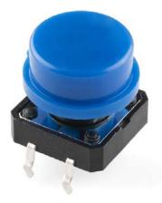
A momentary push button closes or completes the circuit only while it is being pressed. The button has four pins, which are broken out into two sets of two pins. When you press down on the button and get a nice "click," the button bridges the two sets of pins and allows current to flow through the circuit.
