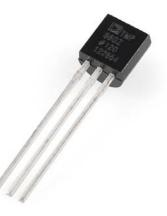
The TMP36 is a low-voltage, precision centigrade temperature sensor. It provides a voltage output that is linearly proportional to the Celsius temperature. It also doesn't require any external calibration to provide
