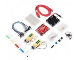
Here are all of the parts in the SparkFun Tinker Kit:
