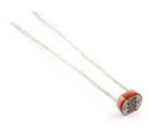
The photoresistor changes its resistance based on the light to which it is exposed. To use this with the RedBoard, you will need to build a voltage divider with a 10K Ohm resistor as shown in the wiring diagram for this experiment. The 101 board cannot read a change in resistance, only a change in voltage. A voltage divider allows you to translate a change in resistance to a corresponding voltage value.
