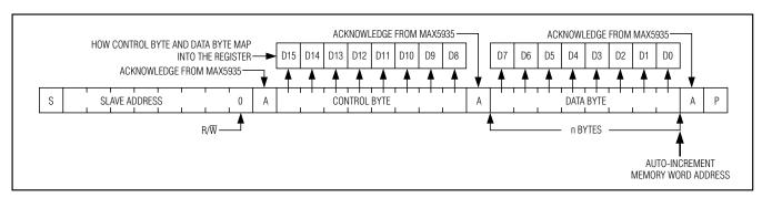
Figure 13. 'n' Data Bytes Received
