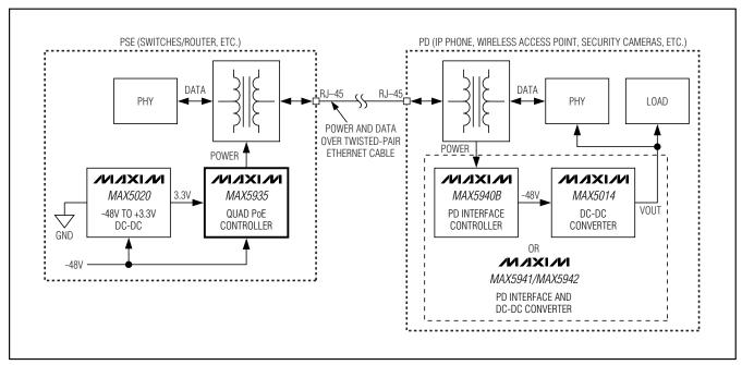
Figure 14. PoE System Block Diagram
