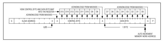
Figure 12. Control and Single Data Byte Received
