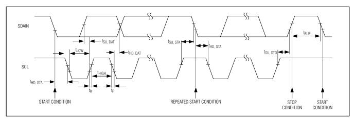
Figure 5. 2-Wire Serial Interface Timing Details
