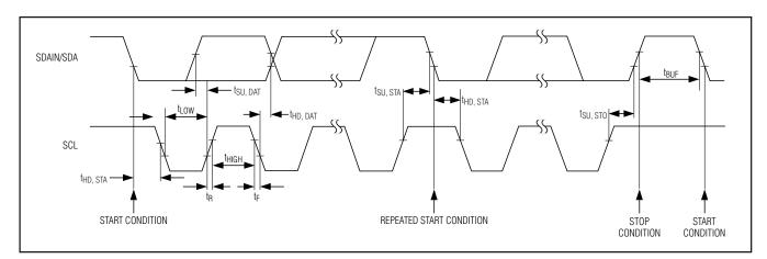
Figure 6. 3-Wire Serial Interface Timing Details
