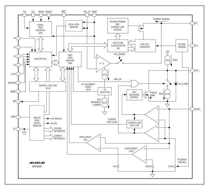
Figure 1. MAX5935 Functional Diagram
