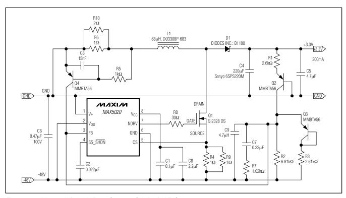
Figure 17. -48V to +3.3V (300mA) Boost Converter Solution for VDIG
