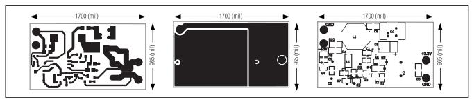
Figure 18. Layout Example for Boost Converter Solution for VDIG
