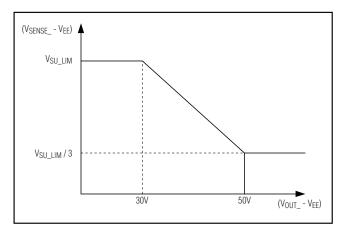
Figure 4. Foldback Current Characteristics
