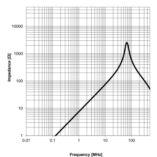
GENERAL TOLERANCE PROJECTION METHOD CREATED CHECKED Würth Elektronik eiSos GmbH & Co. KG **EMC & Inductive Solutions** KaS BMoe DIN ISO 2768-1m Max-Eyth-Str. 1 74638 Waldenburg **WE-MAIA SMD Power Inductor** Tel. +49 (0) 79 42 945 - 0 ORDER CODE www.we-online.com 78438334012 eiSos@we-online.com DATE (YYYY-MM-DD) BUSINESS UNIT REVISION STATUS PAGE 001.004 Valid 3/7 3012 2017-04-17 eiSos **WÜRTH ELEKTRONİK**
