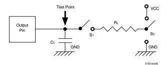
Figure 4. Output Load
