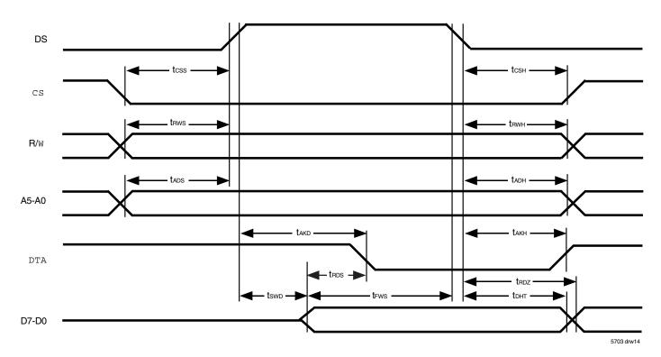
Figure 10. Processor Bus
