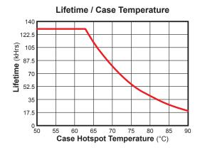
**Note:** The area under the life-temperature curve represents where the driver has highly reliable operation within specification. Driver performance may drift out of published specifications as the hours of operation exceed the curve at a given temperature. Higher operating temperatures increase the chances of a failure to function. Other electrical, mechanical and environmental factors affect driver lifetime but are not represented in this calculation.
