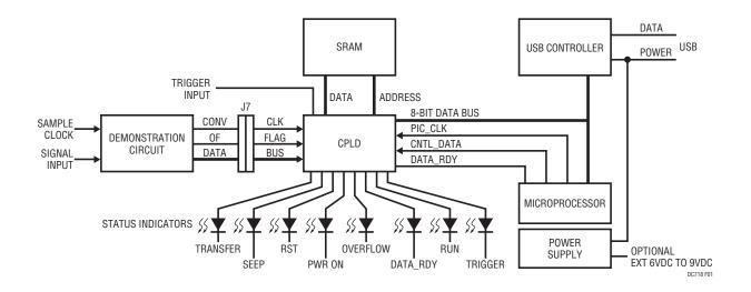
Figure 1. DC718 Block Diagram
